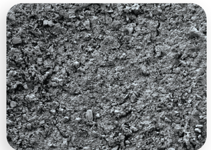
SEM shows glazed porcelain surface after one-minute treatment with Pulpdent Porcelain Etch Gel. Note the microscopic tags in the porcelain surface.
